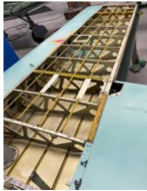
Top from left: the smoking gun - three popped rivets and some bulging of the skin; skin removed; exfoliation corrosion visible. Right: severe corrosion just outside the fuel bay.
