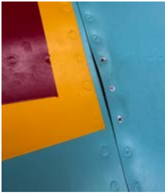
Top from left: the smoking gun - three popped rivets and some bulging of the skin; skin removed; exfoliation corrosion visible. Right: severe corrosion just outside the fuel bay.
