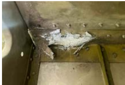
Top from left: the smoking gun - three popped rivets and some bulging of the skin; skin removed; exfoliation corrosion visible. Right: severe corrosion just outside the fuel bay.
