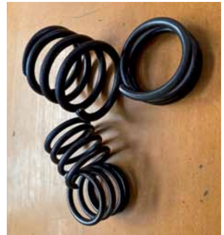
Broken PA-38 valve springs – note the surface corrosion.
