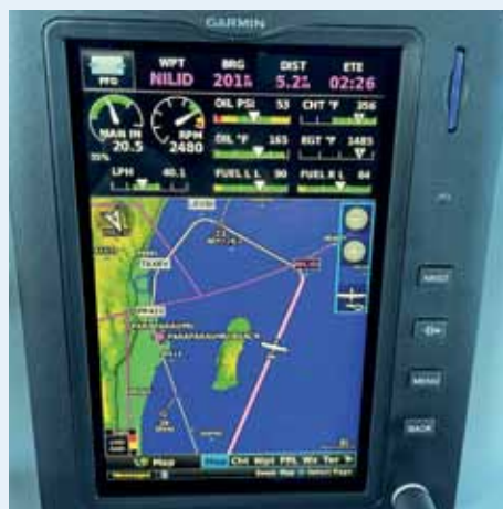
Standard arrival from the north into NZPP for runway 34 with ADS-B showing other aircraft.
