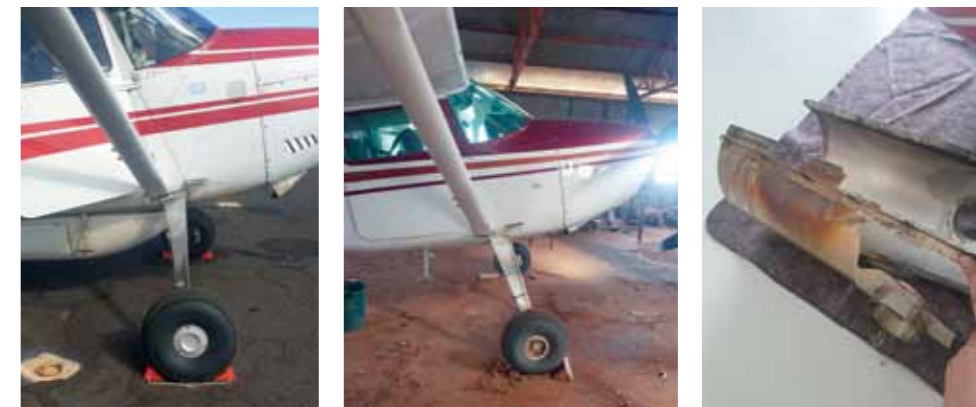
At Charlesville, eastern Australia, Cracker Macdonald pointed out that the landing gear was on the wrong way round (shown at left, compared to the right way, in the centre). Right: a fragment of the exhaust shroud that disintegrated over the Tasman, handed to Tom after touchdown at Kerikeri.
