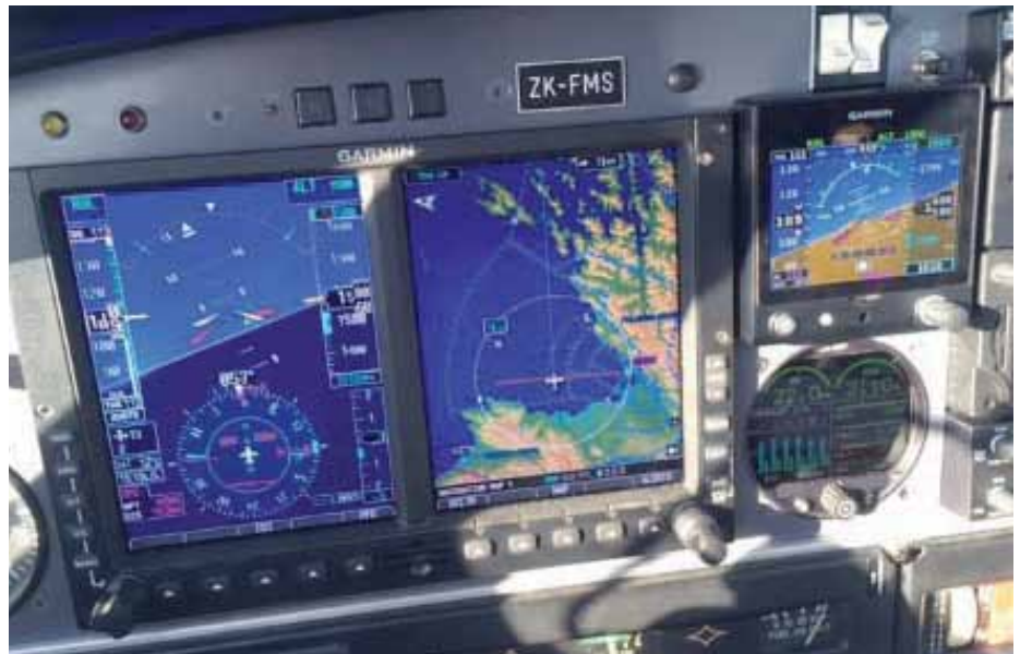
Wings are level, but the G500 has the roll pointer to the left while the G5 has it to the right.
