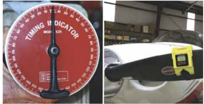
Achieving accurate ignition timing with an old-fashioned 'flowerpot' timing indicator (at left) is almost impossible. Always use a modern digital inclinometer. Inaccurate ignition timing can lead to engine damage.
