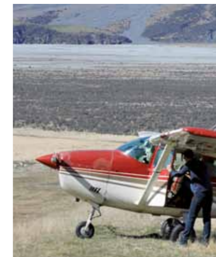
For landings off airfield, make sure the oleo is adjusted to the mid to upper range.
