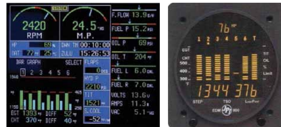
When doing a mag check, focus primarily on your digital engine monitor, not your tachometer. A non-firing spark plug or faulty ignition lead affects only one cylinder; a faulty mag affects all.
