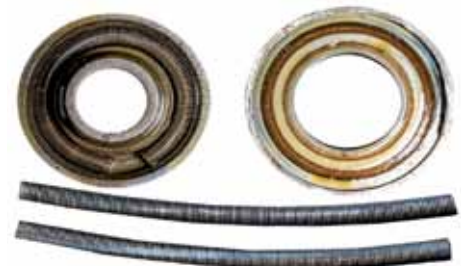
Continental rotocoil disassembled, showing the garter spring (top). Two garter springs, one in good shape, the other badly worn (bottom).
