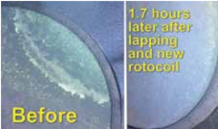
Badly burned exhaust valve, and the same valve 1.7 hours after the valve was lapped in place and the failed rotocoil replaced.
