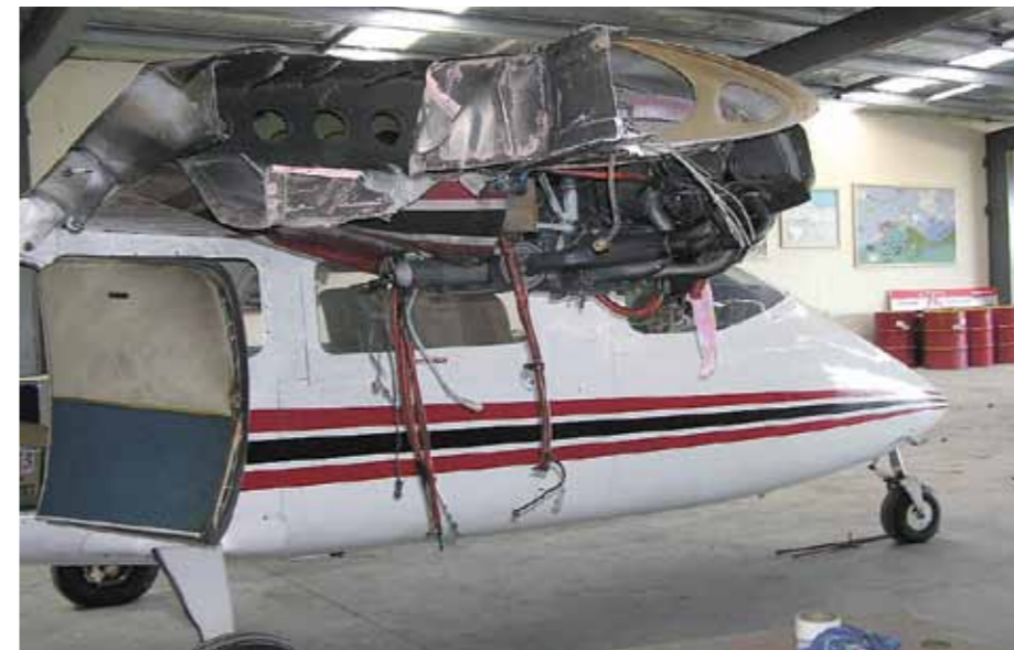
Left: Serious injury can result, as in the case of this Partenavia, when refuelling by jerry can. Metal, appropriately arranged, will ground the static charge that builds up on plastic.
