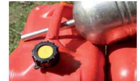
Left: Serious injury can result, as in the case of this Partenavia, when refuelling by jerry can. Metal, appropriately arranged, will ground the static charge that builds up on plastic.
