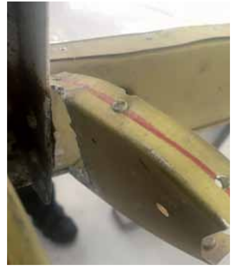
Some examples of the corrosion found in the 1954 Piper Cherokee, including completely rotted out riblets.
