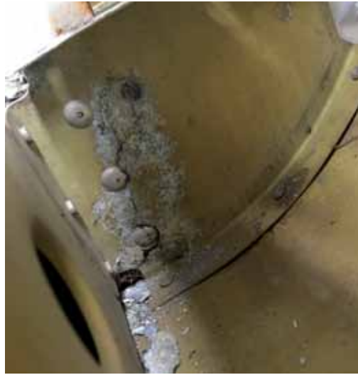
Some examples of the corrosion found in the 1954 Piper Cherokee, including completely rotted out riblets.
